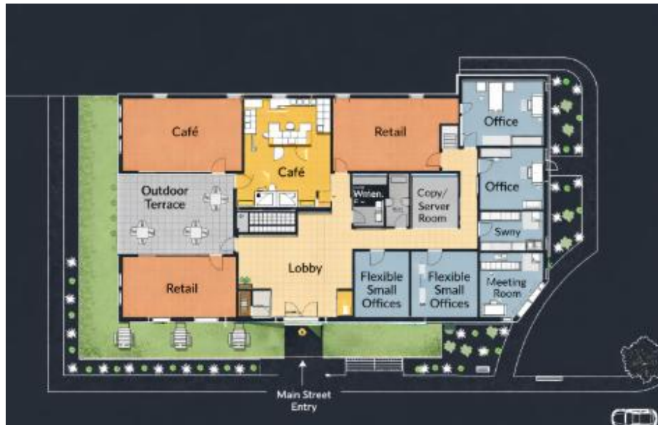
Figure 6. Floor Plan — Core location, Personalized areas and flexible tenant layout.
